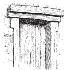
HK00230 Doorpost and lintel
